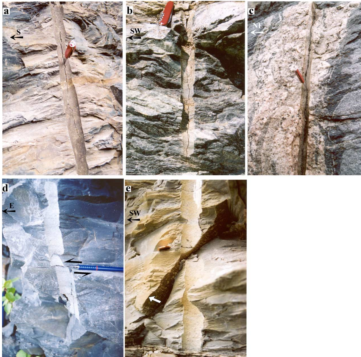
Fig. 2. Examples of axial fractures observed in the concave remains of boreholes along road-cuts and quarries in Finnmark: (a) western Finnmark (SW Altafjord); the strike of the axial fracture is N113°E; (b) central Finnmark (SE Laksefjord); the strike of the axial fracture is N140°E; (c) eastern Finnmark (near Kirkenes), the strike of the axial fracture is N130°E. Examples of borehole offsets found along road-cuts: (d) western Finnmark (SW Altafjord); the offset here is ~1 cm towards N119°E along a plane orientated at N037°E 14°W; (e) central Finnmark (SW Porangerfjord), the offset is ~1.5 cm towards N128°E along a plane orientated at N134°E 58°S.
